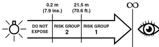
The luminaire should be positioned so that prolonged staring into the luminaire at a distance closer than 21.5 m is not expected.
